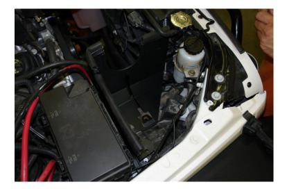
Step 8. Time to install the sheet metal partition. Drop the partition down into the void of the old air box. You will see the tabs where the partition will bolt into place.
