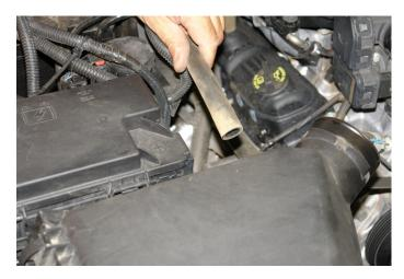
Step1. Remove crankcase vapor return line from airbox.
