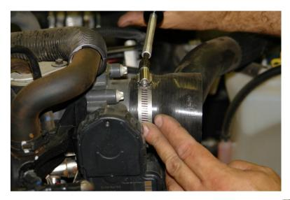
Step 5. Install new rubber reducer adapter
