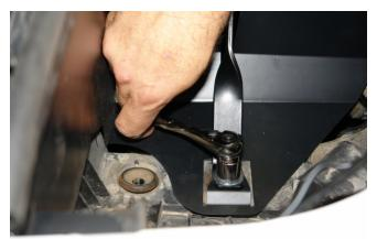
Step 9. As the partition is installed, install the tube support bracket to the rubber mount on the fender as shown, and swing down the air tube into place. Bolt the end of the support bracket to the intake tube.
